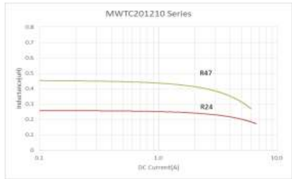
Inductance vs. DC Current Characteristics
