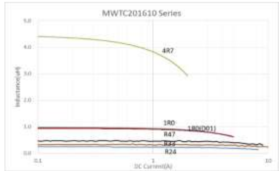
Inductance vs. DC Current Characteristics
