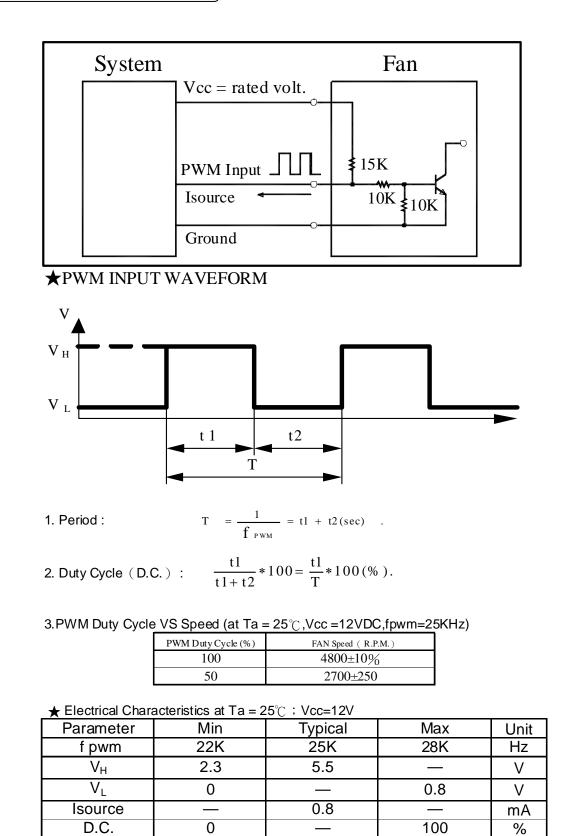
\* The speed is default to be maximum if PWM input pin is unconnected.
