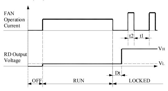
★Electrical Characteristics : (at Ta =  $25^{\circ}$ C , Vcc = 5V)
