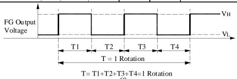
$\Gamma = T1 + T2 + T3 + T4 = 1 \text{ Rotation}$   $T = \frac{60}{\text{rpm}}$
