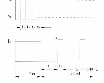
3rd wire signal Run : Square Wave Locked : VH or VL
