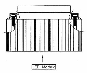
Assembly direction of customer's LED Module
