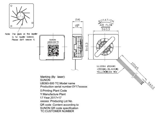
Sunon standard sample exclude the connector. If there is any request for connector, please advise in advance. About recommend connector, SUNON recommend the following models for SUNON Mighty Mini Fan/Blower: 1.(JST) SUR series connector: 02SUR-32S / 03SUR-32S / 04SUR-32S.
