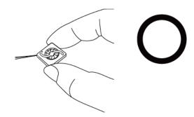
Don't pull fan with lead wires.
