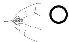
Don't pull fan with lead wires.
