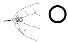
Don't pull fan with lead wires.
