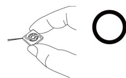
Don't pull fan with lead wires.
