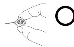
Don't pull fan with lead wires.
