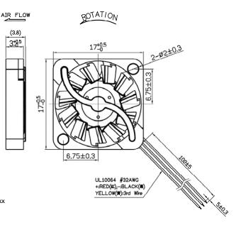
Sunon standard sample exclude the connector. If there is any request for connector, please advise in advance. About recommend connector, SUNON recommend the following models for SUNON Mighty Mini Fon/Blower: 1.(JST) SUR series connector: 02SUR-32S / 03SUR-32S.
