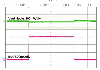
Load Transient Vin=5V / Vout=3.3V / Iout=0.01~1.5A Ch2-Vout ripple, Ch4-Iout
