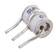
Gas discharge tubes (GDT) use noble gasses enclosed in ceramic tubes to provide an alternate circuit path for voltage spikes. The ceramic envelope and with nickel connectors allow for high loads and Surging offers products that function at 20KA,40KA,50KA,60KA,100KA&150KA.The breakdown voltages of the devices have a wide range (up to 20% tolerance). Major applications are high frequency telecommunication lines, stations, security systems, HID and high quality Surge Protection Devices (SPD).
