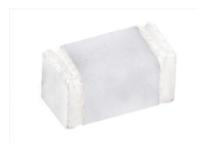
Gas discharge tubes (GDT) use noble gasses enclosed in ceramic tubes to provide an alternate circuit path for voltage spikes. The ceramic envelope and with nickel connectors allow for high loads and Ruilon offers products that function at 20KA,40KA,50KA,60KA,100KA&150KA.The breakdown voltages of the devices have a wide range (up to 20% tolerance). Major applications are high frequency telecommunication lines, stations, security systems, HID and high quality Surge Protection Devices (SPD).
