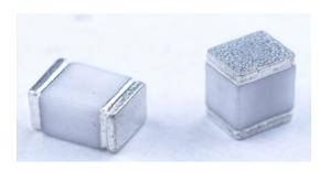
Gas discharge tubes (GDT) use noble gasses enclosed in ceramic tubes to provide an alternate circuit path for voltage spikes. The ceramic envelope and with nickel connectors allow for high loads and Ruilon offers products that function at 20KA,40KA,50KA,60KA,100KA&150KA. The breakdown voltages of the devices have a wide range (up to 20% tolerance). Major applications are high frequency telecommunication lines, stations, security systems, HID and high quality Surge Protection Devices (SPD).
