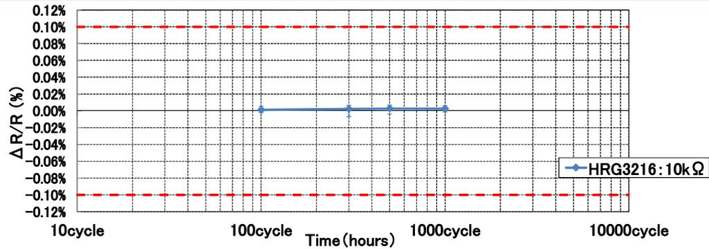
High Temperature Exposure at 155°C with no power
