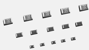
Resistors with high power in small size are realized as 1/3W for 2.0×1.25mm(0805) size, 1/5W for 1.6×0.8mm(0603) size and 1/6W for 1.0×0.5mm(0402) size.
