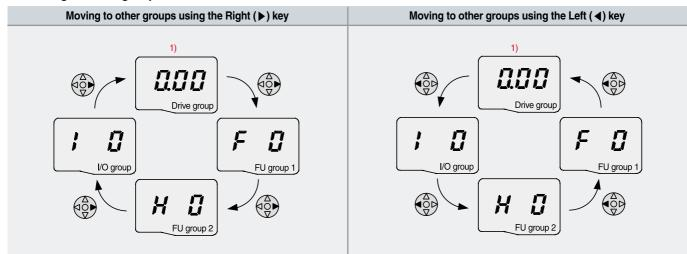
1) Target frequency can be set at 0.0 (the 1st code of drive group). Even though the preset value is 0.0, it is user-settable. The changed frequency will be displayed after it is changed.
