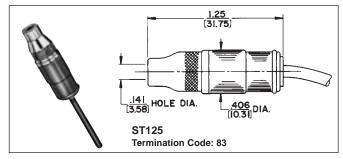
Special Cable: We will build assemblies on cable furnished by you, up to .160" (4.06 ram) outside diameter—or on cable we purchase to your specifications. Jacket must have temperature rating of 60° C minimum.
