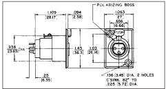
Studio quality black and gold Q-G $^{\circ}$  receptacle with black housing and gold contacts is designed for low/stable contact resistance and withstands corrosion where highest quality is required for recording and broadcast studio equipment, consoles, and other applications.
