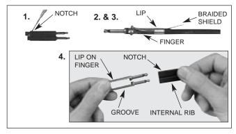
4. ASSEMBLY: Align grooves in fingers with internal handle ribs and insert fingers into rear of handle. Push fingers in until lips or rear of fingers snap into notches on handle.
