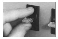
Grasp fingernail slots on opposite sides of escutcheon and snap out. Next, grasp lever and pull lever assembly free. Insert switch into panel hole.
