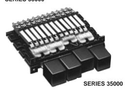
Specify 1 to 18 stations (non-illuminated) with a large selection of mechanical functions, choice of pushbuttons, and up to 6 poles of switching per station. Plungers are on .625" (15.88 mm) centers and are made from .050" (1.27 mm) x .187" (4.75 mm) steel. A square black pushbutton, A592, is supplied with each station. A wide variety of special mechanical functions, features and accessories are also available.
