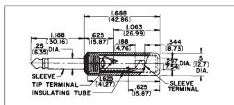
No. 280 typical – shown with solder lug terminals, cord clamp and shielded handle.
