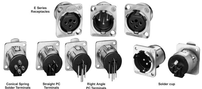
E Series Q-G® Receptacles are available with quick release inserts. Quick insert release is accomplished by turning screw lock from front of insert. Insert can then be removed from the rear. For PC board applications, insert can be removed/assembled to the housing while soldered to the PC board.
