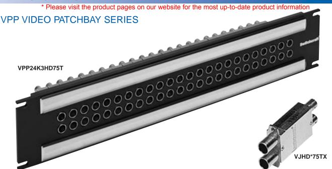
The VPP Series video patchbays offer a wide variety of options for video patching. The HD Series meets SMPTE 292M specifications for high definition video signaling, covering a bandwidth range from DC to 2.4GHz. The SD Series is perfect for serial digital, with a bandwidth from DC to 1.75GHZ. Both come in either terminated or non-terminated, 24 or 26 jacks, 1.75" or 3.5" heights.
