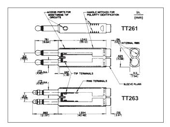
TT263: 6-circuit plug consists of two electrically-independent 3-conductor fingers with black handle. Can use single or dual cables for two electrically-independent 3-conductor fingers or common tip, ring and/or sleeve circuits.
