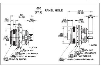
Front of panel mount; 2 through 5 pins (male) or 2 through 5 contacts (female). Also 2-, 3- and 4-contact insert with 3 shunted (N.C.) contacts. Mounting locknut (Part Number SL01), lockwasher (Part Number SL02), and flat washer (Part Number SL03) supplied.
