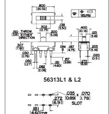
RECOMMENDED PC BOARD LAYOUT (Component Side)
