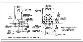
**RIGHT-ANGLE** SHIELDED RECEPTACLE for printed circuit board mounting
