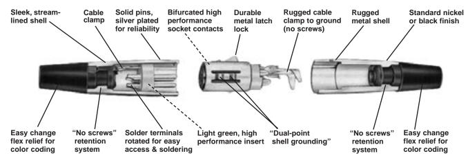
QGP connectors (3 contacts only) feature Vel-Tone® non-reflective finish, gray TPR flex relief and plated pins/contacts for the most demanding applications.
