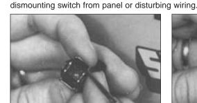
For color filters, use fingernails or small screwdriver to remove. Gently lift (don't pry) up under edge of filter until it "pops" out.
