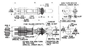
MAXIMUM PANEL THICKNESS SERIES 3000 .094" (2.39mm) SERIES 13000 .250" (6.35mm)
