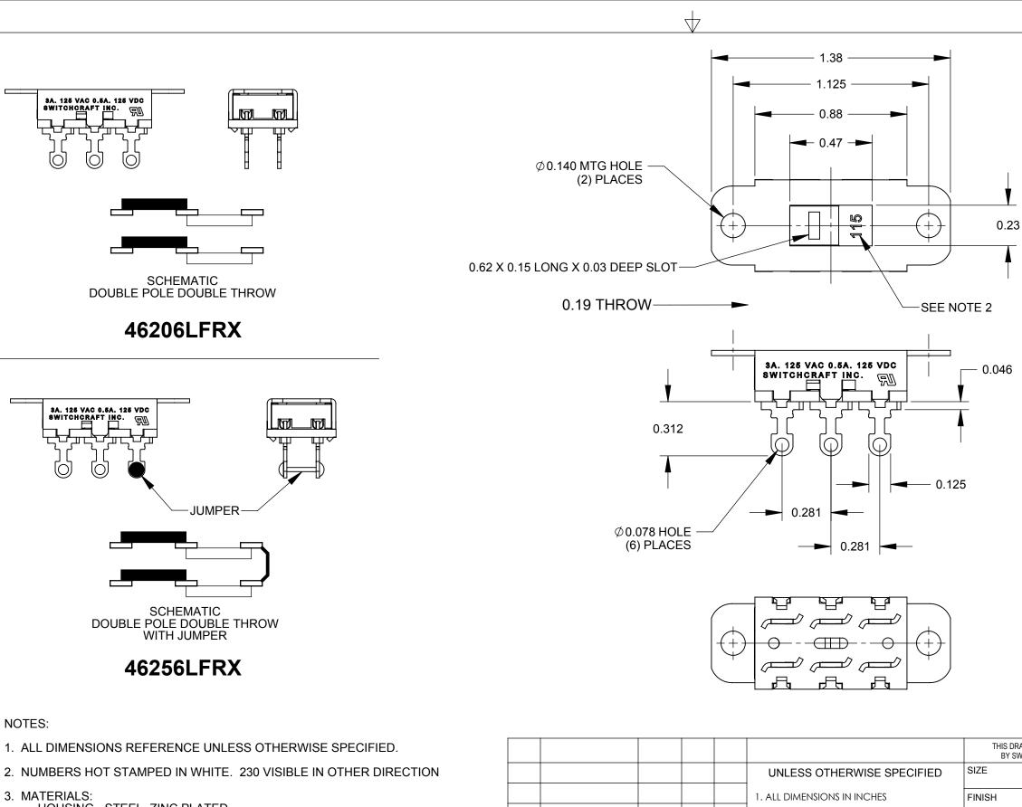
HOUSING - STEEL, ZINC PLATED **BUTTON - THERMOPLASTIC, BLACK** TERMINALS & CONTACT SLIDER - BRASS, SILVER PLATED **TERMINAL BOARD - PHENOLIC**
