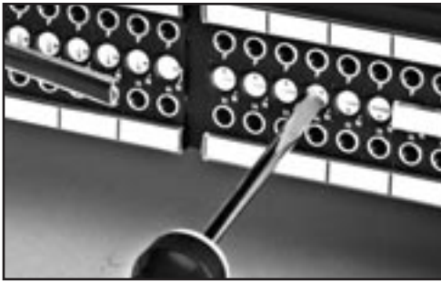
Center Strip Removes For Normalling Access
