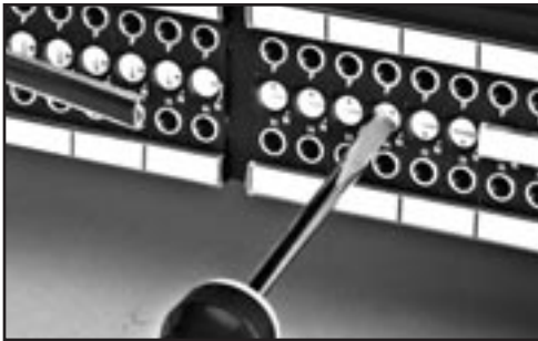
Center Strip Removes For Normalling Access
