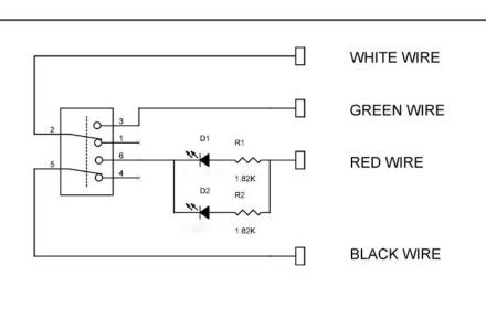
SCHEMATIC CIRCUIT 1A WITH LEDs
