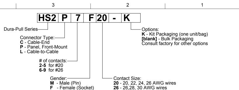
Refer to HS2C SERIES drawing for mating Cable-End connectors. Refer to HS2L SERIES drawing for mating Cable-to-Cable connectors.
