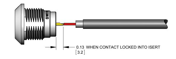
6. ALIGN AND INSTALL FINISHED CONNECTOR INTO PANEL CUT-OUT. TIGHTEN HEX NUT TO A MAXIMUM OF 40 IN-LB [4.5 Nm].
