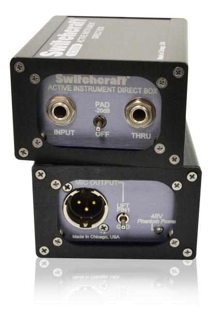
A 48V phantom powered instrument direct box designed to quietly preserve the tone of the world's finest musical instruments. The SC800A is ideal for converting the unbalanced outputs of passive musical instruments such as acoustic guitar and bass to balanced, mic level signals that can be connected to audio consoles and mic preamps. Precision engineered active circuitry provides extended reach and superior audio fidelity for professional audio engineers and musicians
