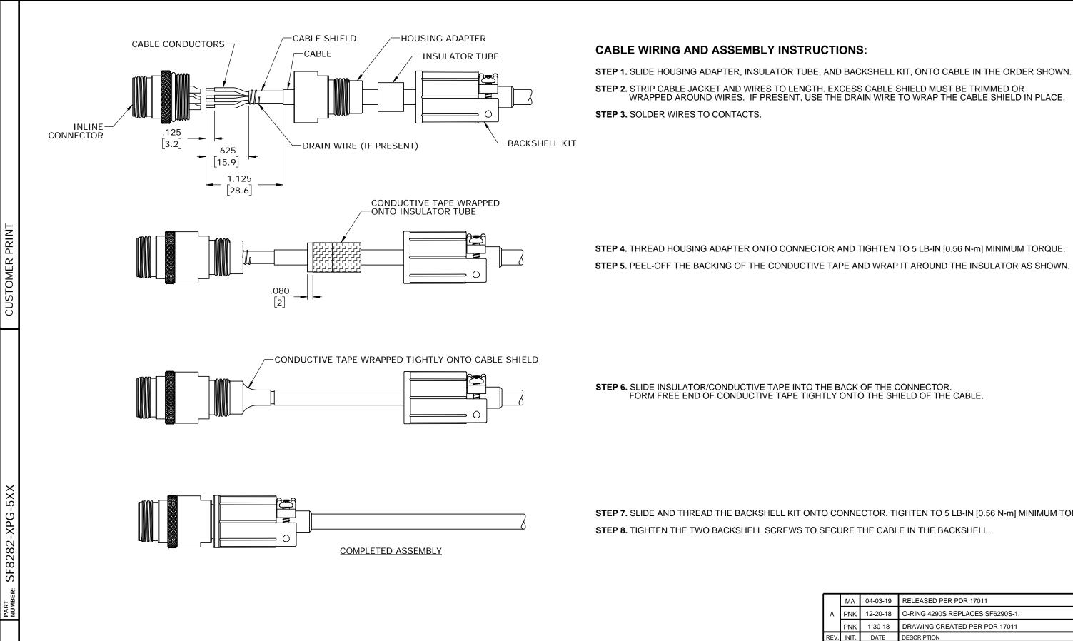
STEP 7. SLIDE AND THREAD THE BACKSHELL KIT ONTO CONNECTOR. TIGHTEN TO 5 LB-IN [0.56 N-m] MINIMUM TORQUE.
