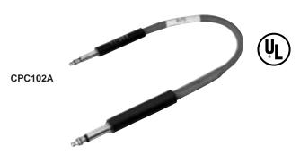
Series CPC Combination Patch Cords provide convenient interconnections between standard telephone-type jacks (3-conductor, .25" inside diameter sleeve) and miniature telephone-type jacks (3-conductor, .173" inside diameter). Series CPC cords are ideal for connection in telephone, data processing and other telecommunication applications where both standard and miniature jacks are available for patching.
