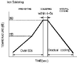
Iron Soldering times: 1 times max.
