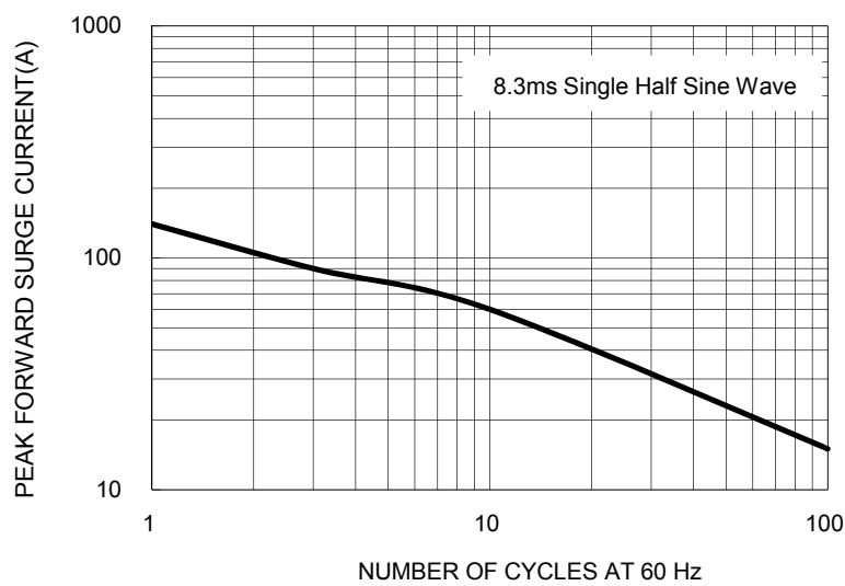
FIG. 3 MAXIMUM NON-REPETITIVE PEAK FORWARD SURGE CURRENT
