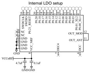
Internal LDO setup with external 32.768kHz X'tal
