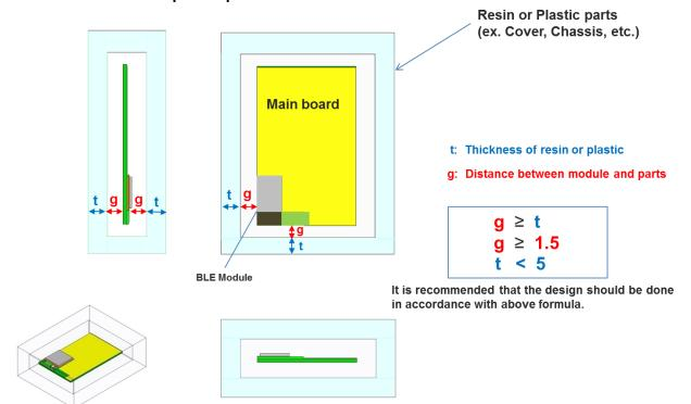
Please do not apply molding over the antenna area of BLE module.
