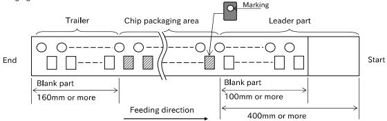
The number of empty compartments in a reel, which shall not appear continuously, must be limited to 2.
