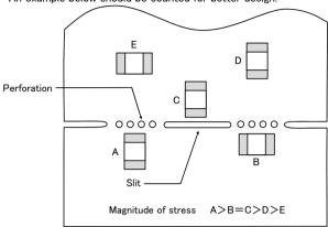
3. When breaking PC boards along their perforations, the amount of mechanical stress on the inductors can vary according to the method used. The following methods are listed in order from least stressful to most stressful: push-back, slit, V-grooving, and perforation. Thus, any ideal SMD inductor layout must also consider the PCB splitting procedure.
