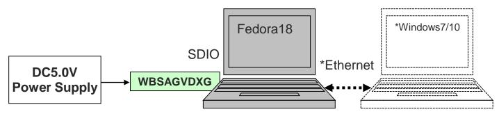
\*To use LABTOOL, PC with Windows7/10 is also required. Each PCs are connected via Ethernet cable.
