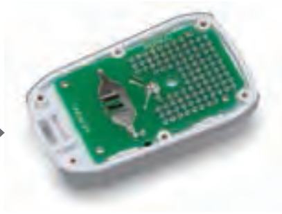
Install the PCB in the top cover
