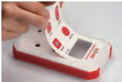
8. Sticking overlay sheet onto enclosure
