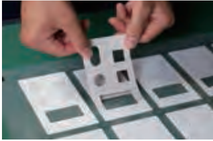
4. Sticking double-sided tape on printed film
