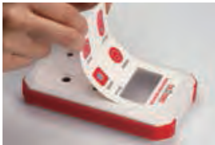
8. Sticking overlay sheet onto enclosure
