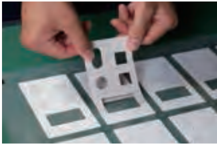
4. Sticking double-sided tape on printed film
