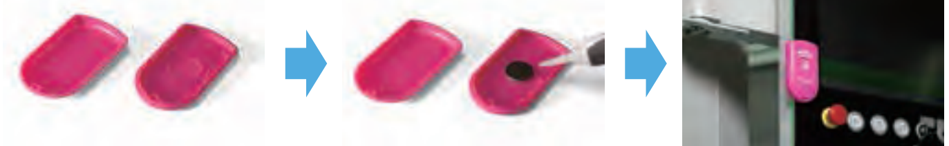
Make recessed pocket on the inside wall.
