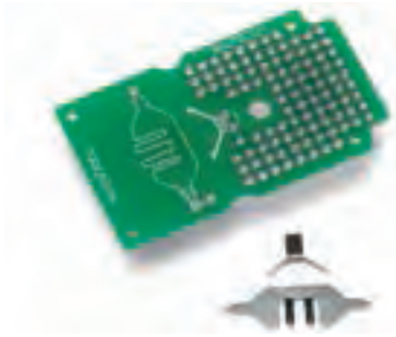
Solder the contacts onto the PCB
