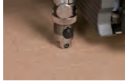
3. Cutting double-sided tape
