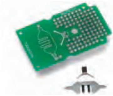
Solder the contacts onto the PCB
