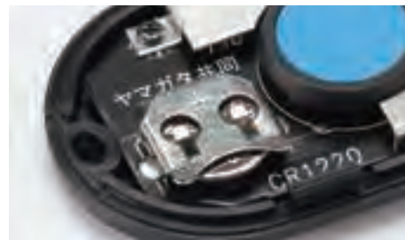
TAKACHI "BK-890" Coin battery holder is used.
