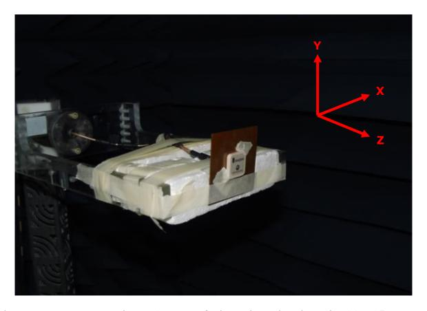
The antenna is measured on a CTIA certified anechoic chamber. The CGIP.25 antenna is put on a 70\*70mm ground plane.
