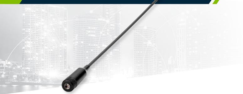
The Meteor FW.80 is a 0dBi 169MHz ISM band 1/4 wavelength monopole flexible whip antenna with omnidirectional pattern optimized in the azimuth for wide coverage range in typical 169MHz applications such as Wireless M-Bus metering. It also finds its usage in remote asset monitoring applications, alarms, paging systems and private mobile radio services.
