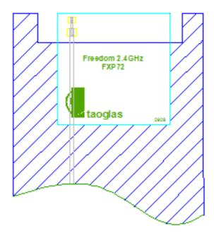
The size of the ground plane used on the testing had a dimension of 40X60 mm, see next figure 14. The antenna was placed in the center of one shortest edge. The antenna was in between the ABS plastic and ground plane, having a clearance of 8 mm. The Antenna was tested into the Satimo system chamber and with a network analyzer. The antenna was also tested on in free space, just the antenna stuck out on the ABS plastic of 1.5 mm of thickness.
