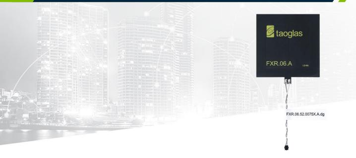
The FXR.06.52.0075X.A is an NFC Ferrite antenna on 75mm twisted pair 28AWG cable with JST connector. It works with specific NFC chips which need to connect via JST ACH connector.
