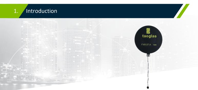
The FXR.07.52.0075X.A is a circular, flexible, NFC (Near Field Communications) antenna for use in mobile devices and other applications such as keycards, payment systems, and boarding passes. The design provides a flexible NFC antenna with 75mm twisted pair 28AWG cable that can be adhered to the plastic enclosure of the device for ease of installation and work with specific 13.56MHz RFID and NFC chips which need to connect via JST ACH connector.
