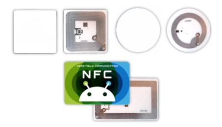
Type 1 tag is based on ISO/IEC 14443A standard and has 512 bytes of memory. Type 2 tag is based on ISO/IEC 14443A standard and has 192 bytes of memory. Type 4 is based on ISO / IEC 14443A 1-4 compliant and has 2K of memory.
