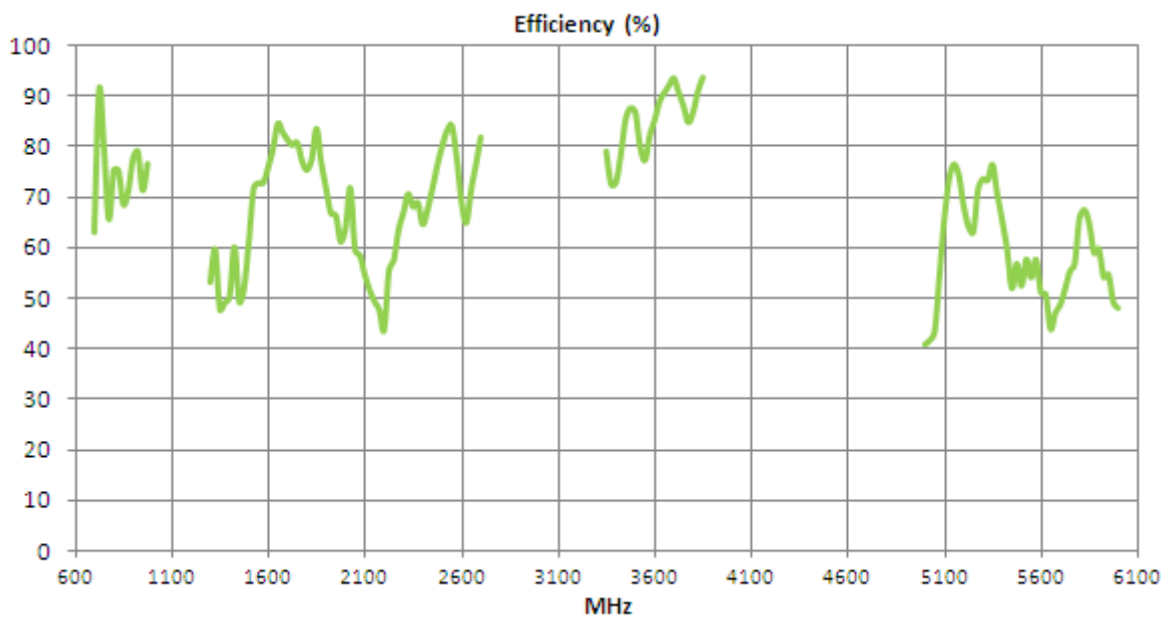
Figure 4. Efficiency of FXUB66 UWB Antenna.
