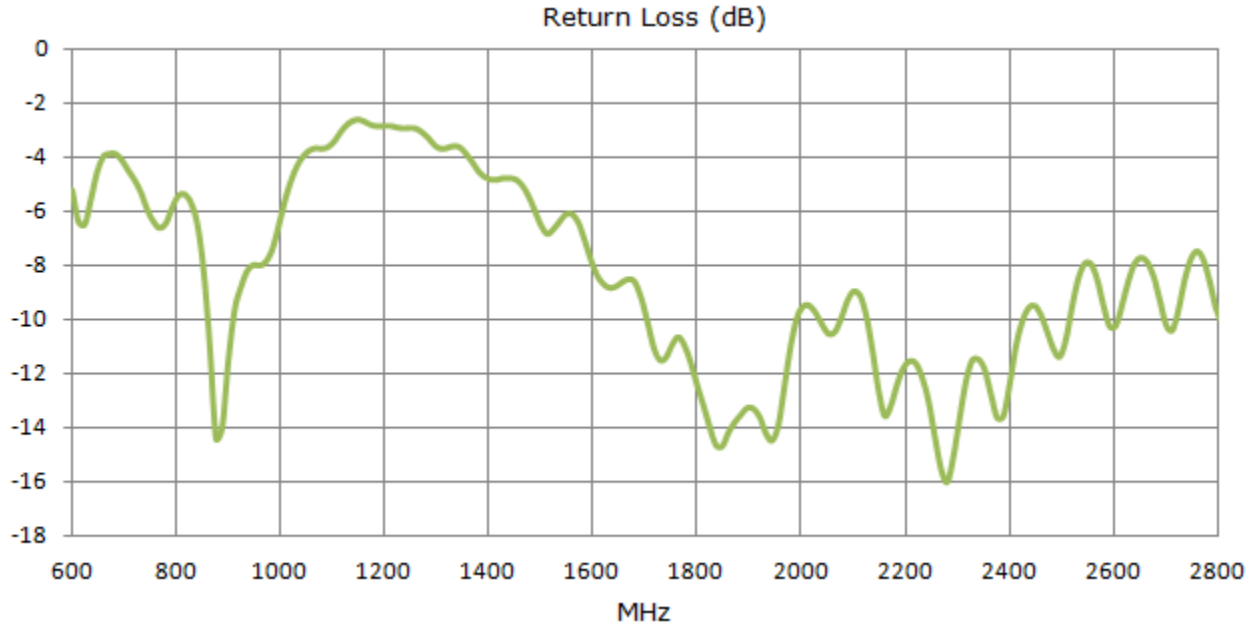
Figure 2. Return loss of G30 Antenna in Free Space
