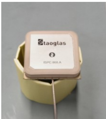
Ground under antenna
